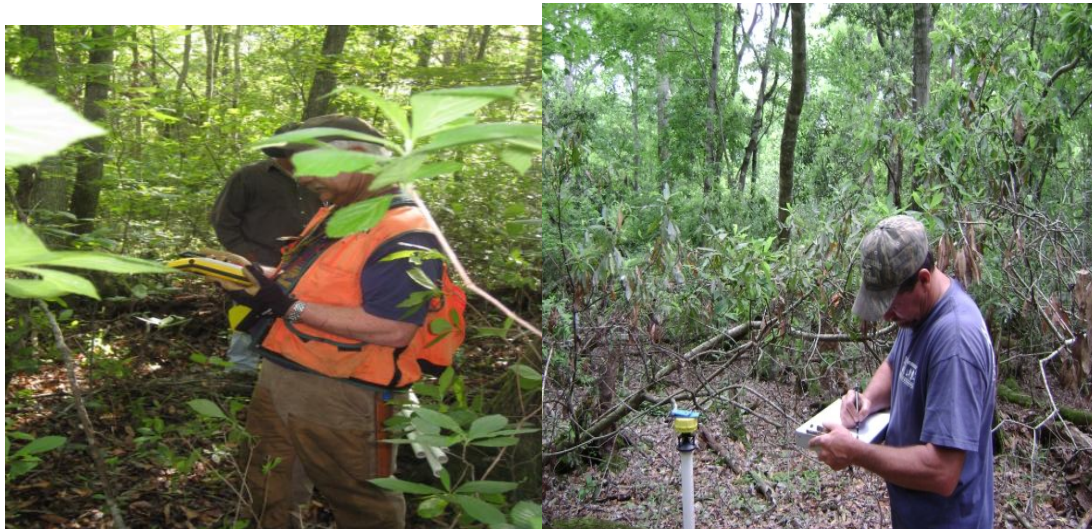
Figure 3 - Recording plot coordinates/data; and DME instrument and pvc pipe at plot center
