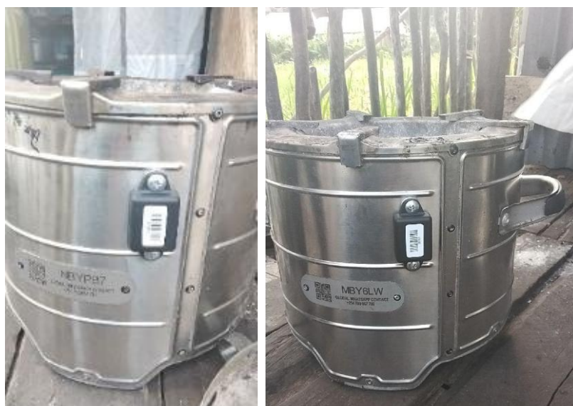
Figure 5 Continuous stove monitors
