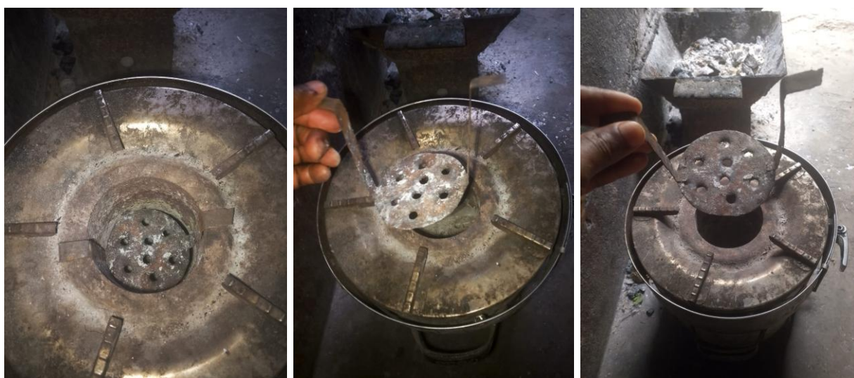
Figure 15 Top view of an improved firewood stove showing a perforated metal grate placed above the combustion chamber, enabling charcoal use. The original stove structure remains unchanged
