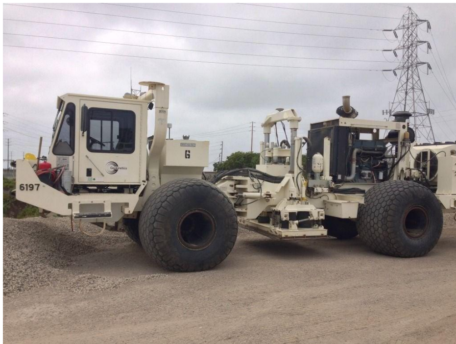
Figure 67. Vibration truck used to perform Seismic analysis.
