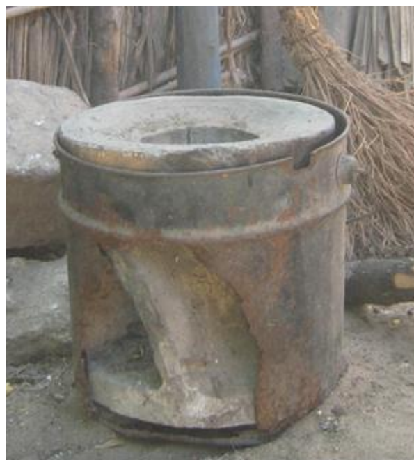
Oli-b stove (&gt;3 years old) not repaired
