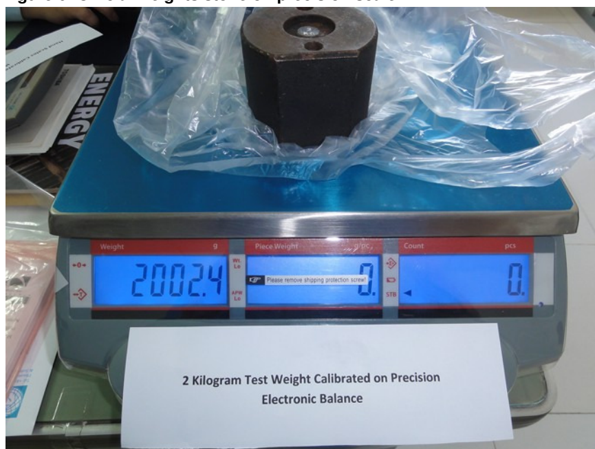
Figure 6: Official weights stone on precision scale
