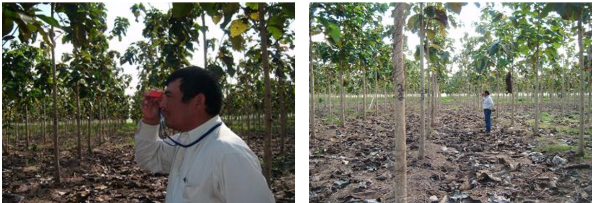
Figure 33: Measuring with a clinometer
