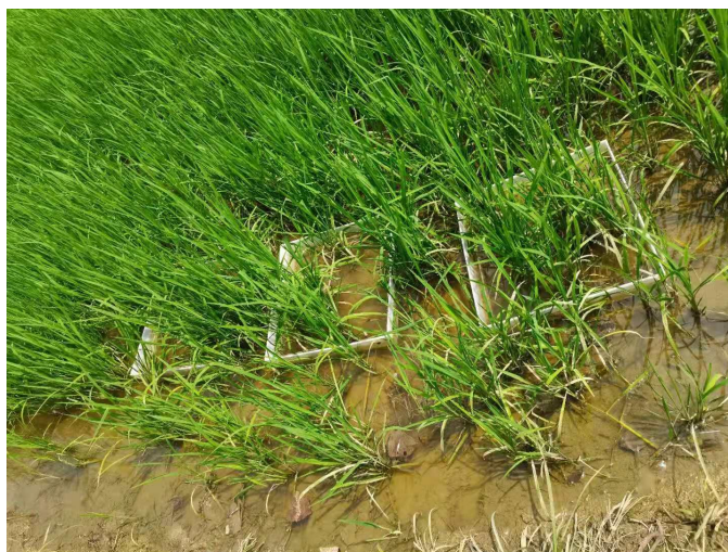
Figure 4-5 The base buried in the reference fields (which covers 4 rice hills)
