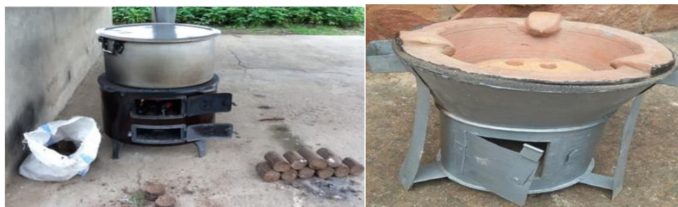
Improved Institutional cookstove with briquettes (left: Turc Medium, right: Matawi)
