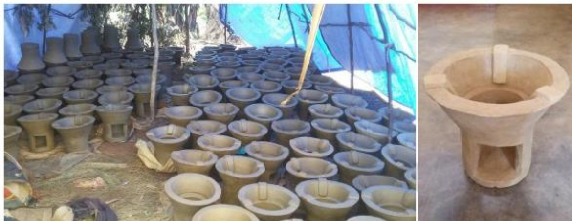
Figure 6 : Drying and final stove inspection for distribution
