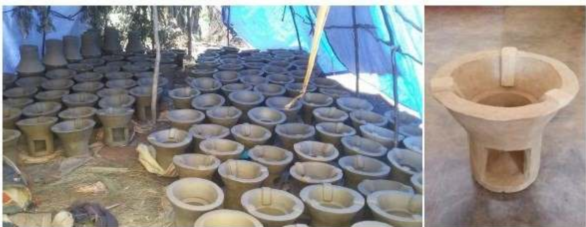
Figure 6: Drying and final stove inspection for distribution
