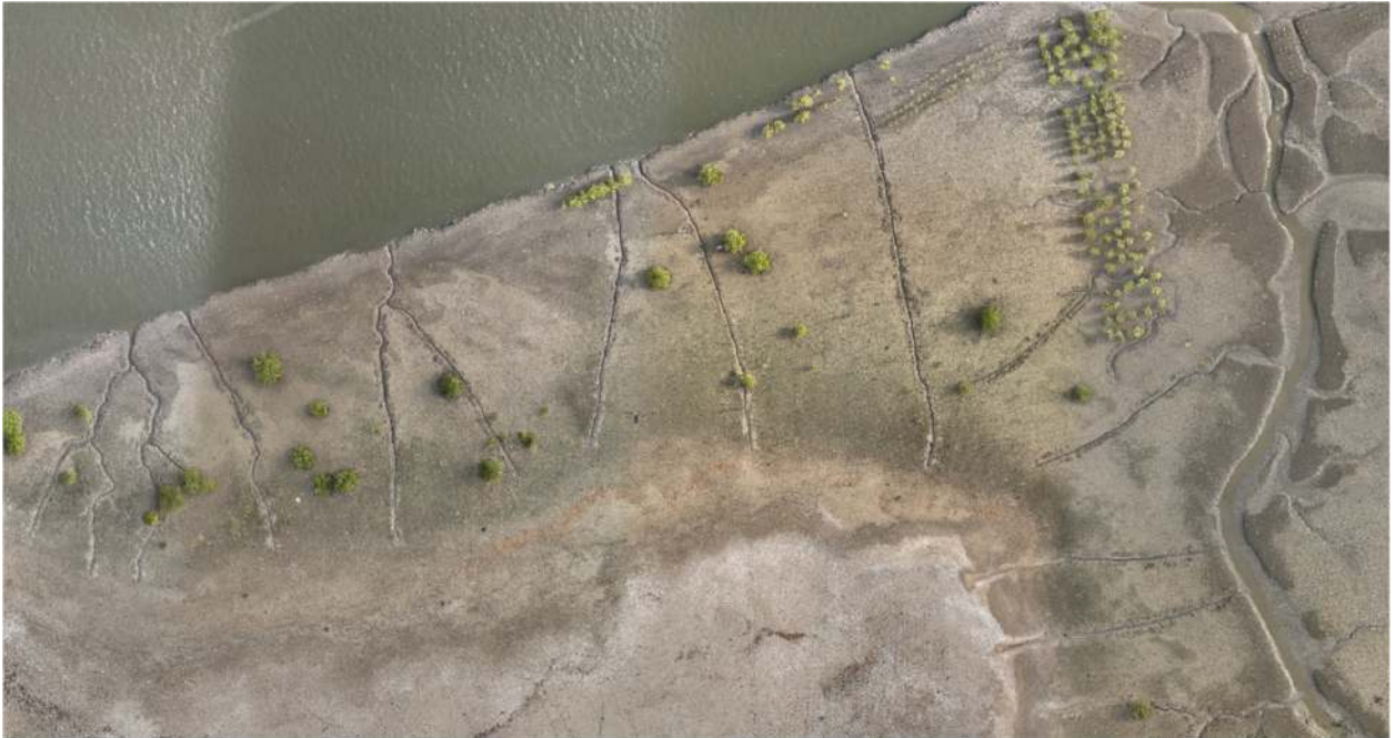
Picture 6. Image of excavation done in Joreng to increase water flow.
