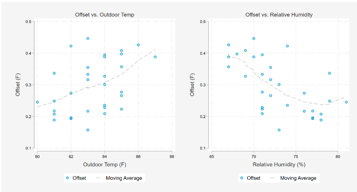
Figure 3: Offset Versus Outdoor Temperature and Relative Humidity (July 2021)
