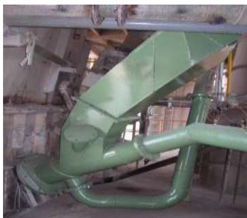
Figure 6: New air feeding system
