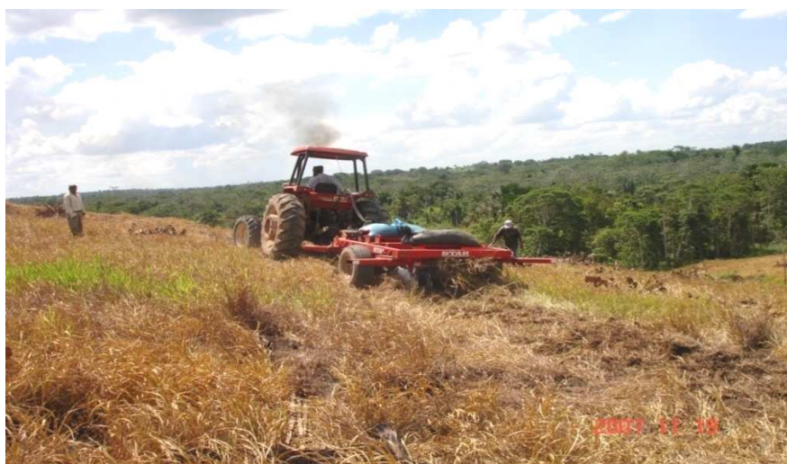
Figure 12 Offset disc ploughing of 1m wide strips along the contour
