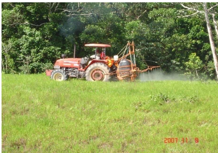
Figure 11 Mowing and herbicide application using tractor mounted sprayers
