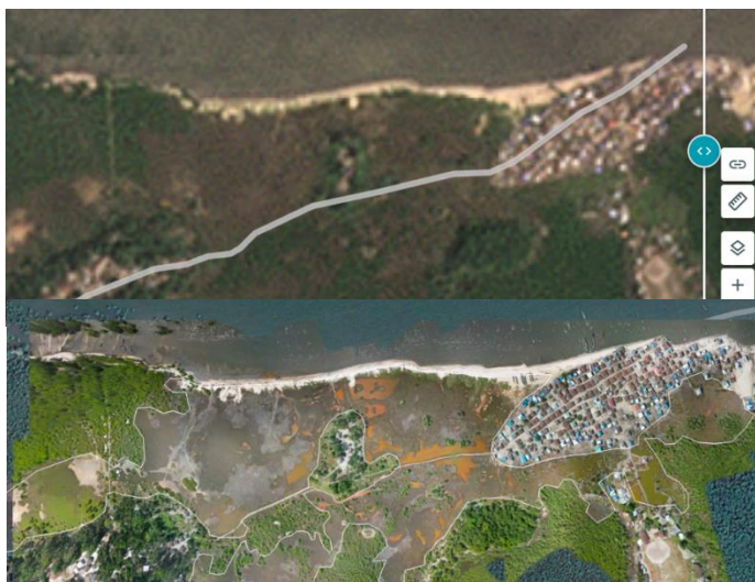
Figure 6: A comparison of Delkin, a community on Sherbro Island, Sierra Leone, as seen by Planet satellite imagery (top) and drone orthomosaics (bottom) in March 2023. The most recent Google Earth imagery of this location is from 2018.
