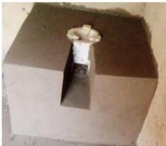
Figure 4: RDIS stove after installation
