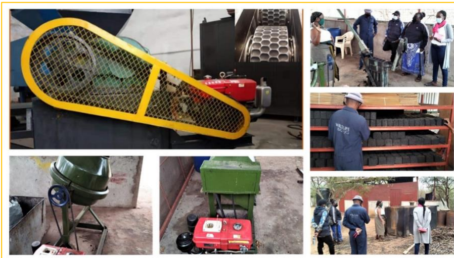
Figure 28: Clockwise L-R: The mechanized briquette press, manual press, eco-charcoal briquettes, improved kiln, grinder and mixer acquired during the M 7 monitoring period
